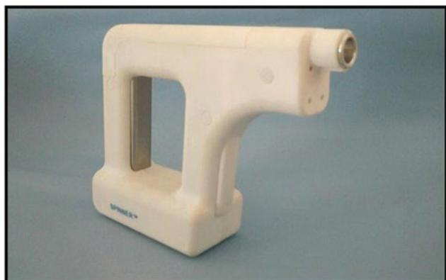
**Figure 1.** Handheld electrospinning device.
